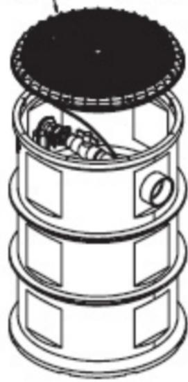
**POLYLOK FULLY ASSEMBLED PUMPING STATION**
