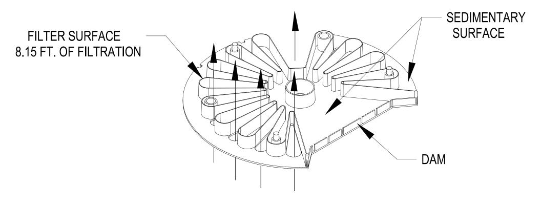
EFFLUENT ENTERS THROUGH THESE OPENINGS IN FILTER PLATES
